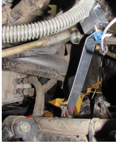
Figure 5: Potentiometer mounted to the ATV steering column for controlling the simulator's steering.
