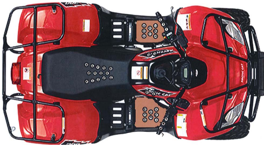
Figure 17: Location of each of the 48 force sensors placed on the ATV. The 8 sensors placed under the handlebars are not pictured.
