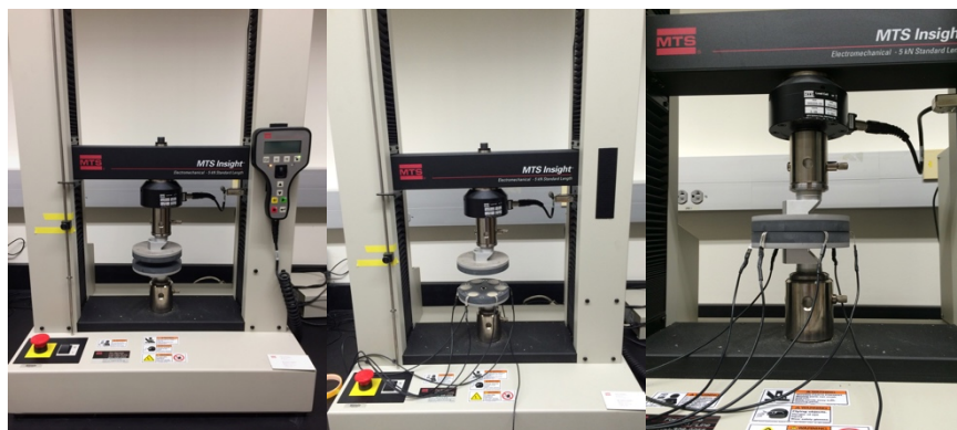
Figure 16: An MTS machine was used with a compression protocol to load the force sensors. Not pictured, pucks were used in final calibration to concentrate the load on each sensor. Sensors were tuned during maximum compression.
